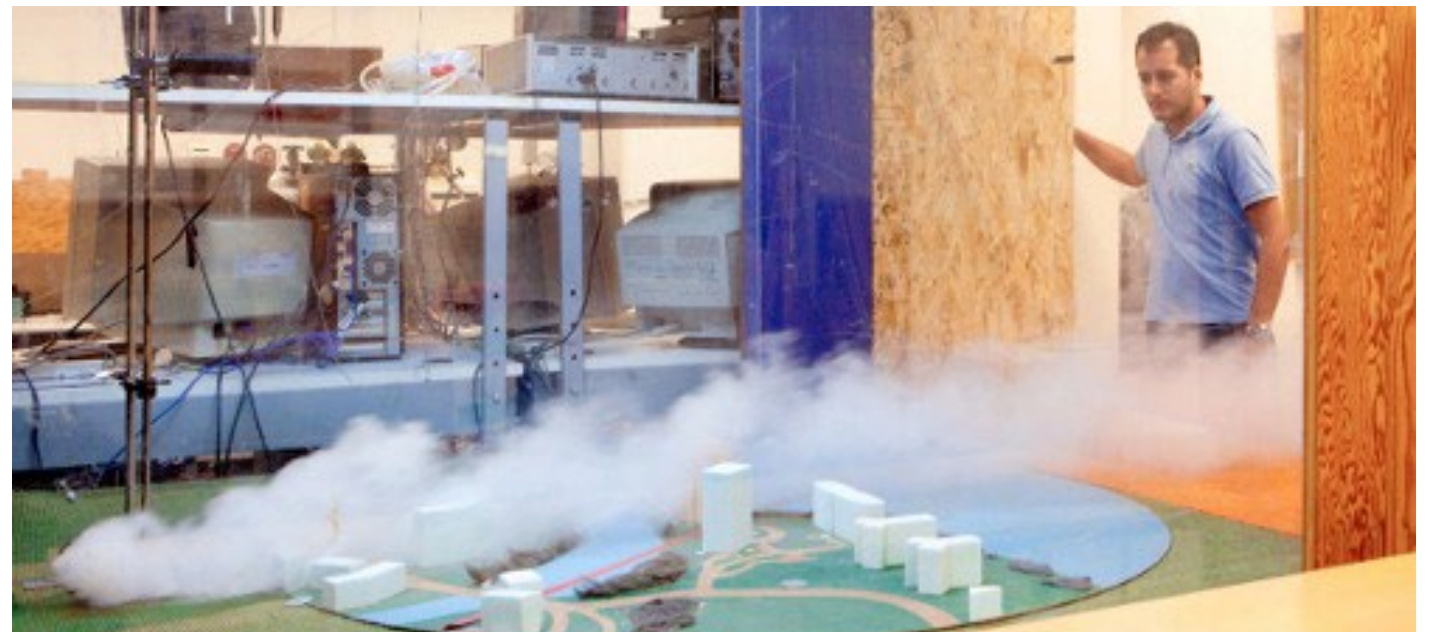
Right: Smoke generated around scaled model buildings inside BLWT for studying contaminant dispersions within an urban environment.
