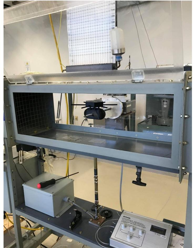
Printed-3D model wind tunnel testing
