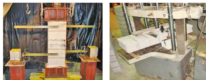
Fig. 1. Tests for obtaining compressive (left) and tensile (right) strength of masonry assemblage
