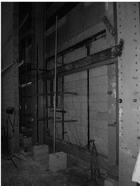
Fig. 5. Typical wall instrumentation
