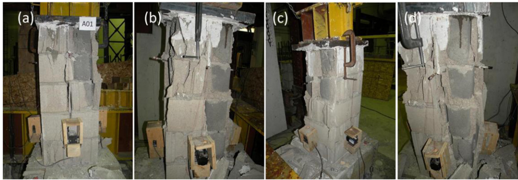
Fig. 9. Observed failure mechanism of the unreinforced boundary element column.
