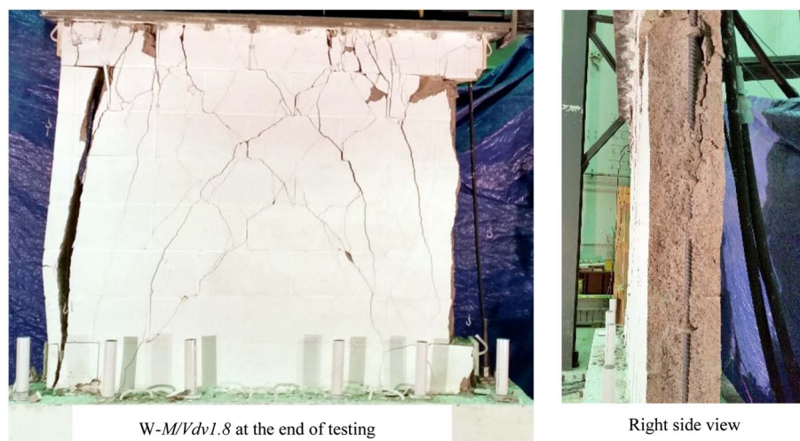
Fig. 21. Final crack pattern of tested Wall W-M/ Vd_v 1.8
