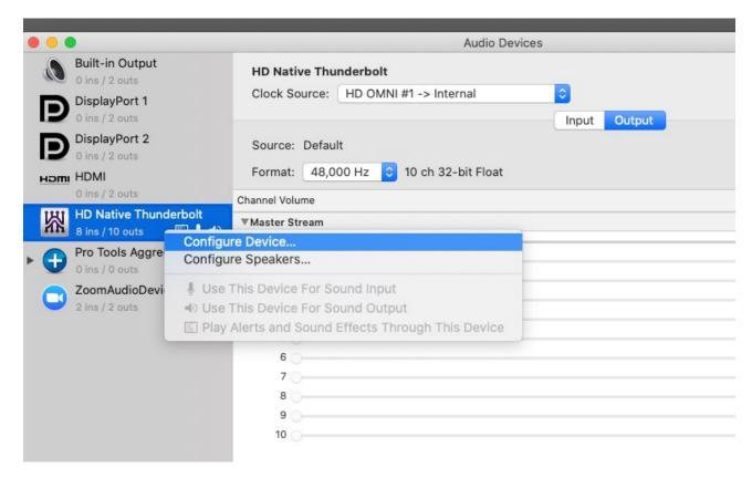
Once an application other than Pro Tools is launched, You should see the HD Native Thunderbolt as an Audio Device in the Audio MIDI Setup software in Applications/ Utilities.
