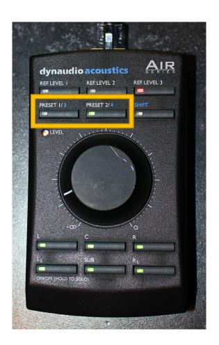
The two PRESET buttons control the volume of the side speakers.
