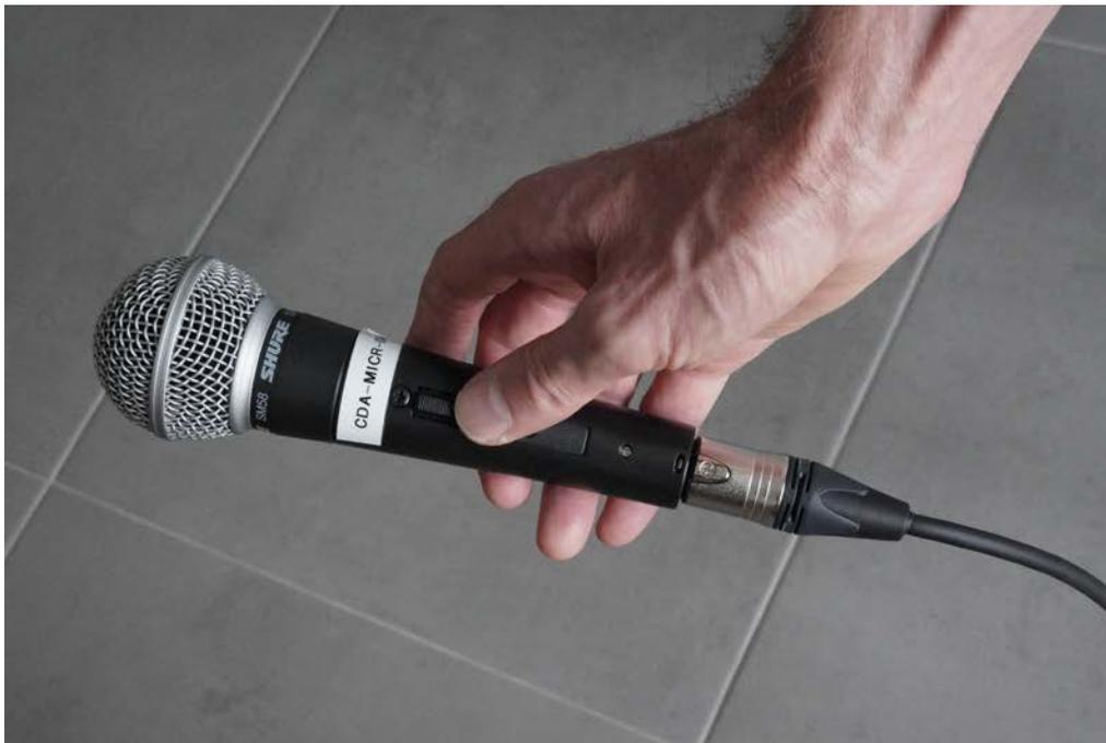
The Shure SM58 is a dynamic microphone. It does not require power to operate.
