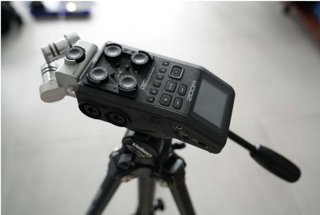
This is the Zoom H6N recorder. The CDA has different models of Zoom recorders with either two, four or six microphone inputs. They all operate with AA batteries.
