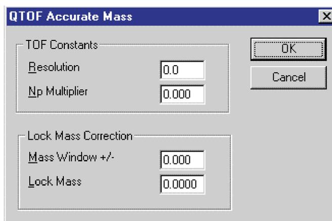
Re-center the data using **Resolution** = 10000 and **Np Multiplier** = 0.7 as below:
