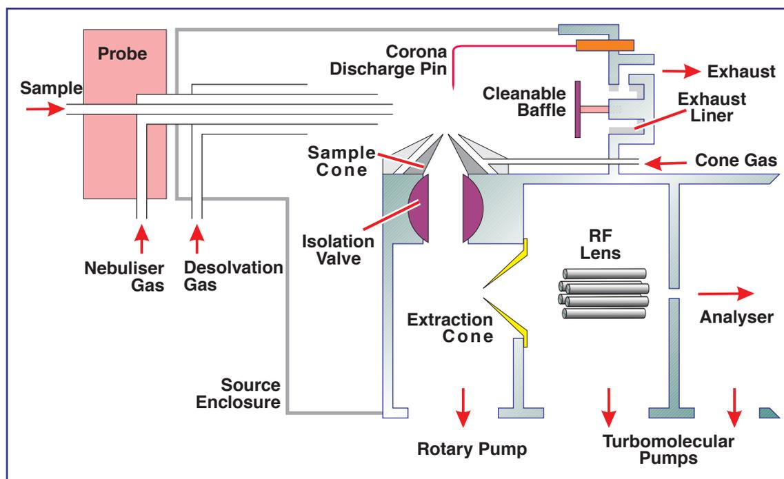
Atmospheric Pressure Chemical Ionisation (APCI) is an easy to use LC-MS interface that produces singly-charged protonated or deprotonated molecules for a broad range of involatile analytes.
