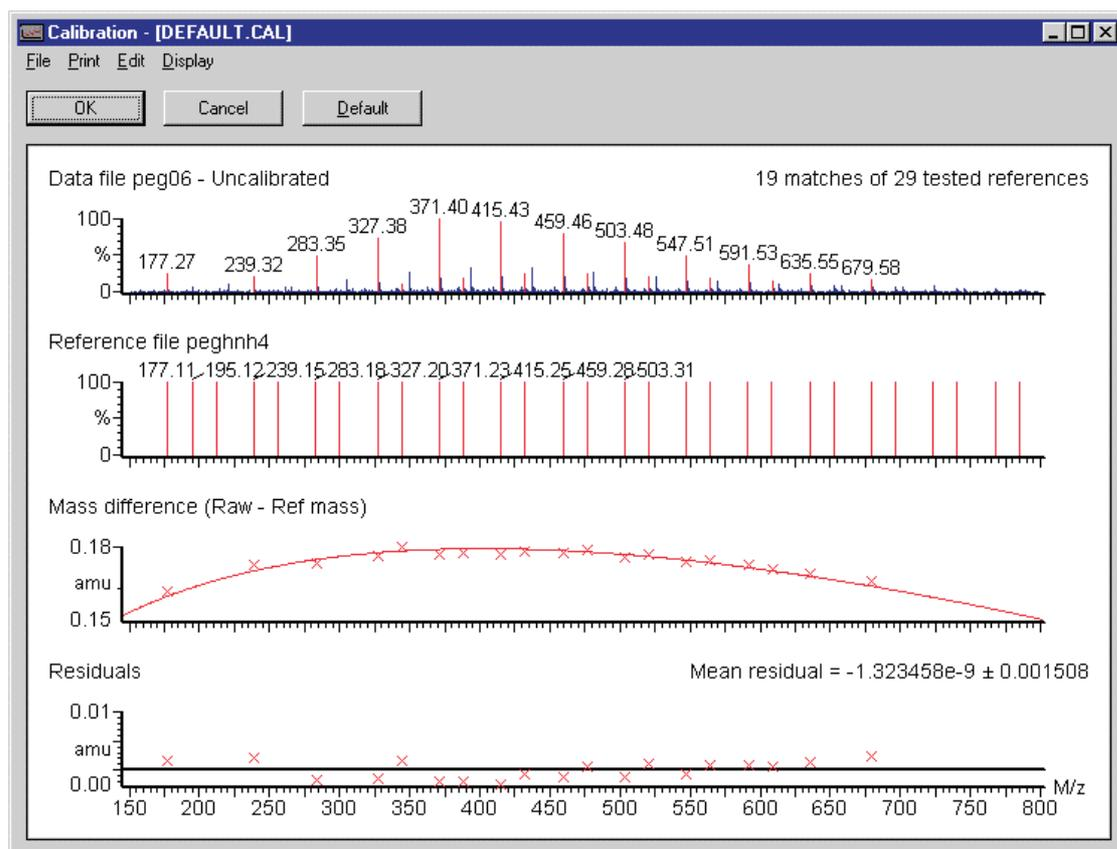
Typical values for **Np Multiplier** will be about 0.7, and the **Resolution** used should be as measured on the instrument at mass 500.
