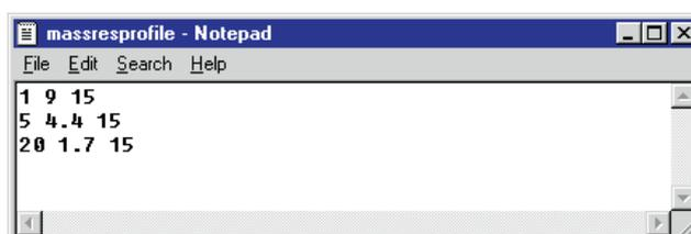
The left most number is the transmission window of the quadrupole followed by the **LM** and **HM Resolution** settings.
