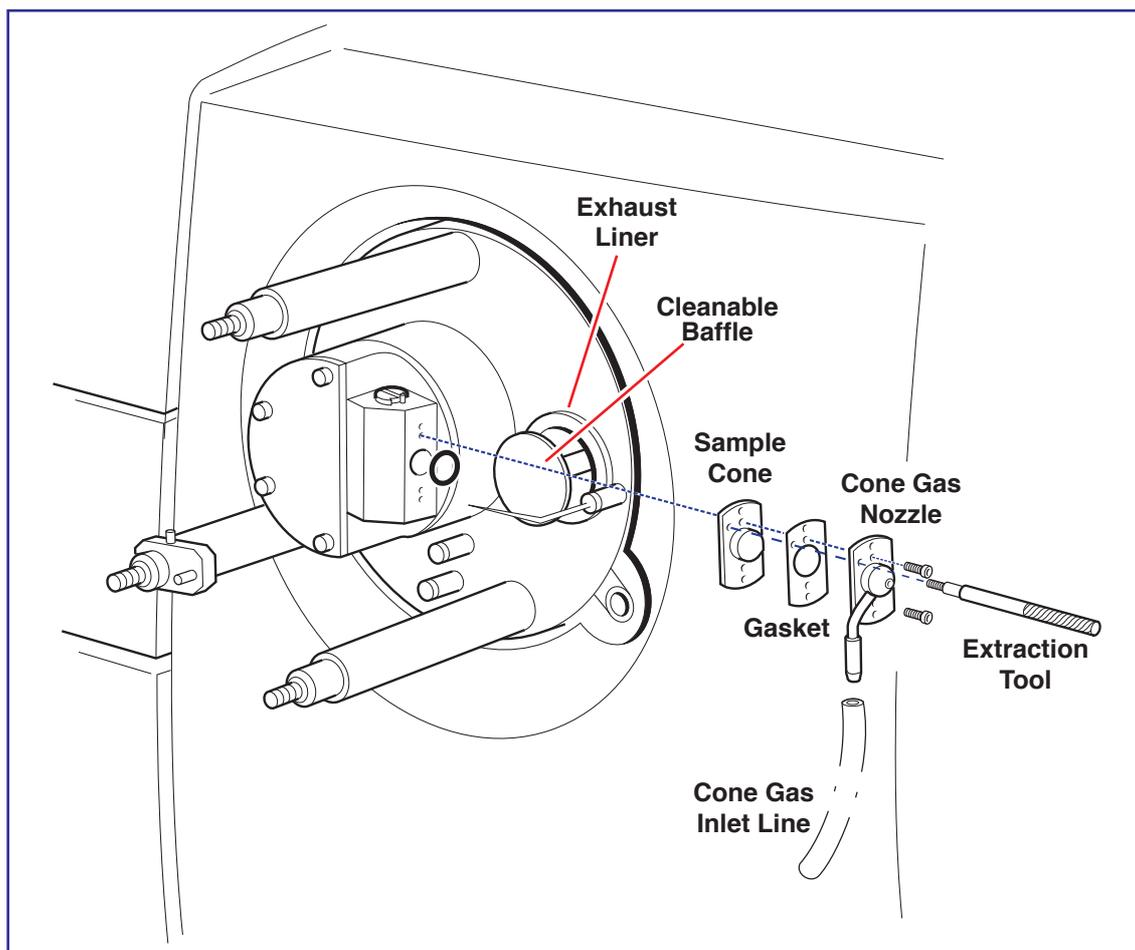
Dry the cone and nozzle using nitrogen.
