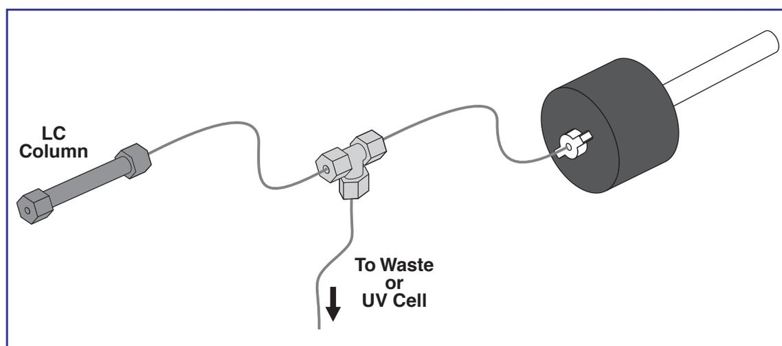
The split ratio is adjusted by increasing or decreasing the back pressure created in the waste line, by changing either the length or the diameter of the waste tube. A UV cell may also be incorporated in the waste line, avoiding the requirement for in-line, low volume "Z cells". As the back pressure is varied, the flow rate at the probe tip should be checked as described above.
