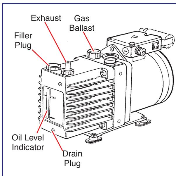
Gas ballasting should be performed routinely on a weekly basis for 30 minutes. If the source is used in the APcI or megafLOW electrospray modes, more frequent gas ballasting is recommended.
