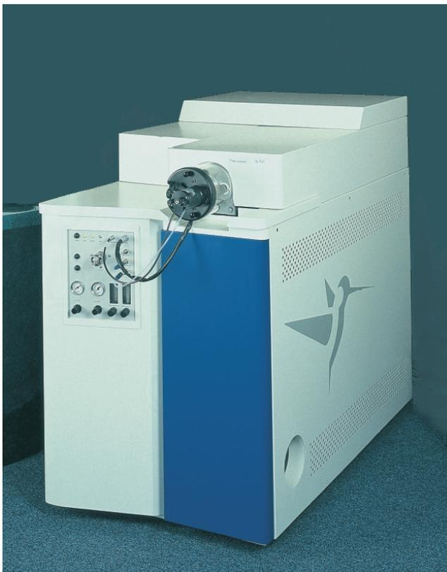
The Q-Tof 2 hybrid quadrupole time of flight mass spectrometer is available with electrospray ionisation (ESI) and atmospheric pressure chemical ionisation (APCI).
