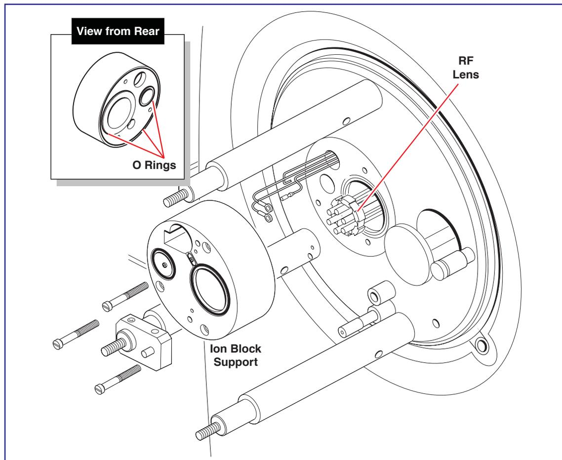
To remove the RF hexapole transfer lens assembly, proceed as follows:
