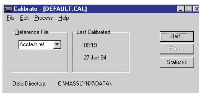
Select the reference file to use (pehnh4.ref will give the correct masses with the sample prepared as described above).
