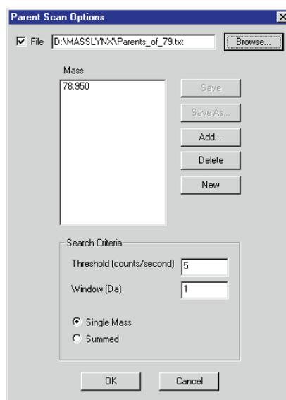
If not, or if a different set of products is to be specified, then a new file can be created using the **New** and **Add** facilities.
