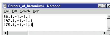
The cursor must be at the end of the last text line (i.e. the last character in the file must not be a carriage return). If precursors are being sought for more than a single product ion then a new line is added for each using the same format as shown. It might be useful to create a Folder in the MassLynx root directory (e.g. Parents) in which to place these files.
