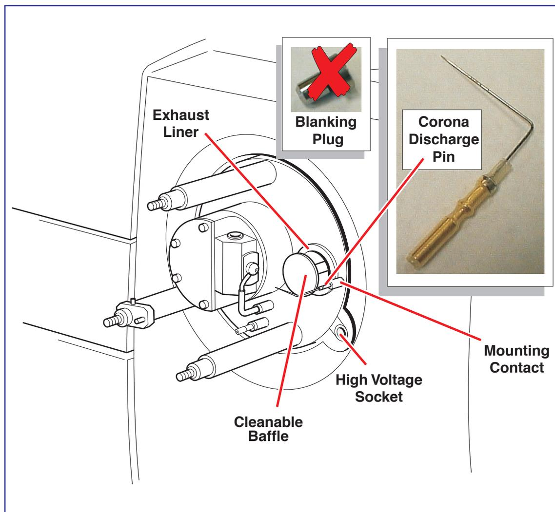
*APcI may be operated with or without the cleanable baffle fitted.*
