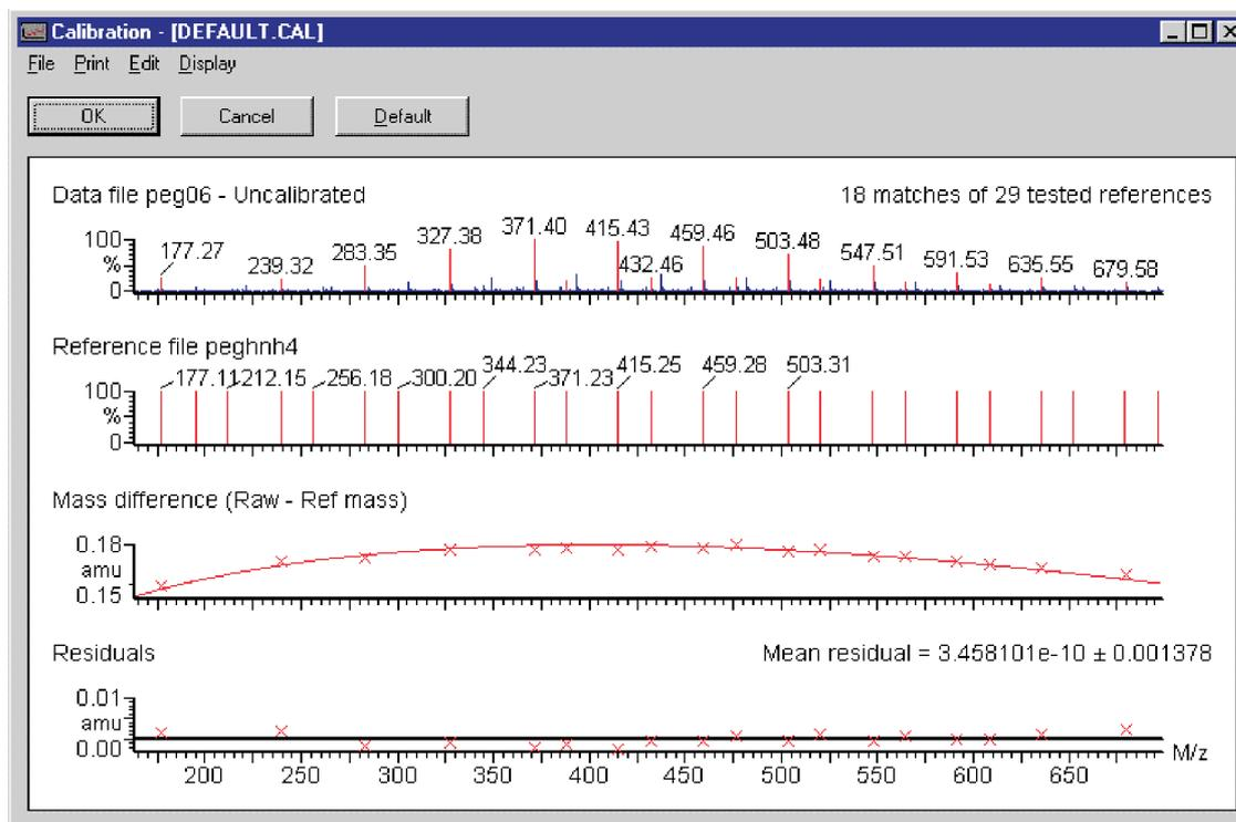
Make sure that the residual errors are all less than 3 mDa. The calibration parameters can be altered by clicking on **Edit** to reveal the box below:
