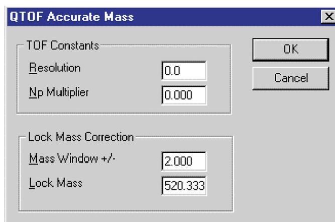
Centering the spectrum with these parameters will force the peak at 520 to be 520.333 exactly and recalibrate the entire mass spectrum.
