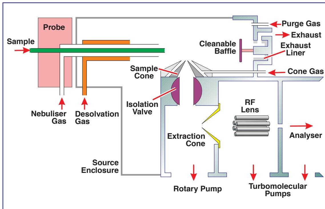
The ESI interface consists of the standard Z-spray source fitted with an electrospray probe. See the following chapter for additional information concerning the optional nanoflow interface.
