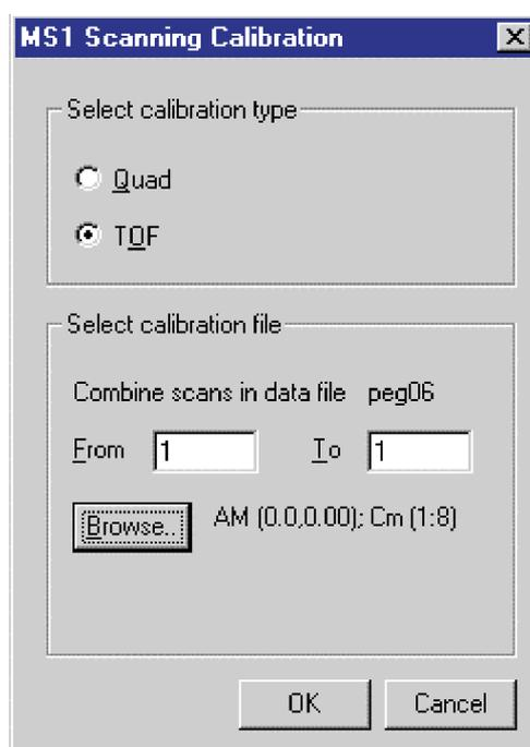
Use the **Browse** option to select the centred spectrum which has been previously saved. In the above example box it is from a data file peg06. Once the spectrum has been selected click on **OK**:
