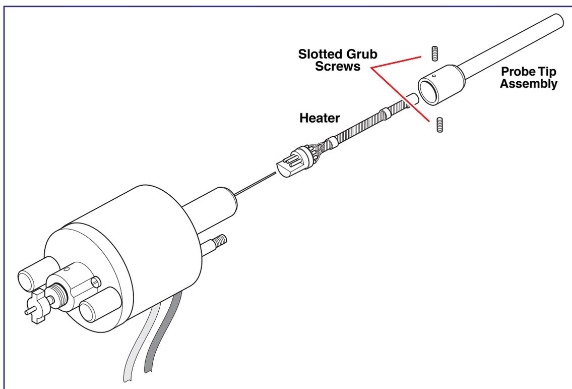
Remove the probe tip assembly by carefully loosening the two grub screws.
