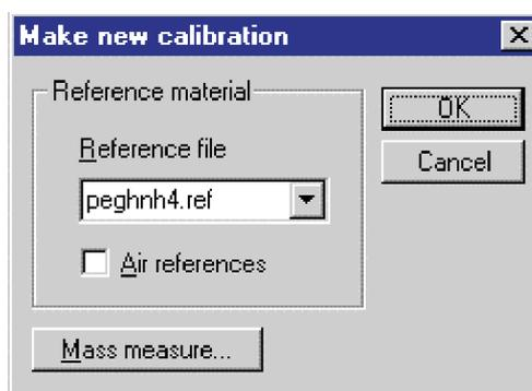
Click on **OK** to reveal the residual errors, whilst making sure that a polynomial of order1 has been selected. The deadtime distortion is revealed as the observed difference between the high and low intensity peaks:
