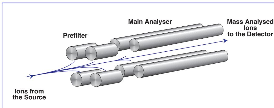
The need to clean the prefilter rods is usually indicated by poor peak shape or loss of resolution (in tuning mode), although other more likely causes, such as contamination of the source should be eliminated first.
