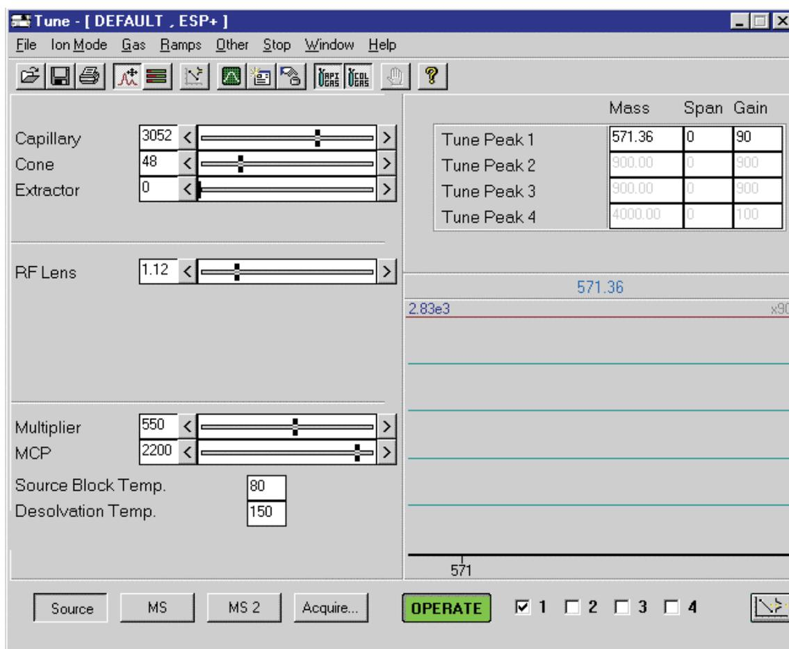
The positive ion electrospray (ESP+) source tuning menu is shown. Suggested tuning parameters are as follows:
