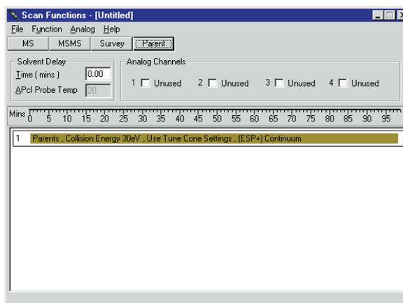
A second function is added by selecting the **Parent** button and the Function 2 Parent Scan window appears. All parameters in this window should be set to be the same as in function 1 except the **Step Mass**, which should be set to 5Da.
