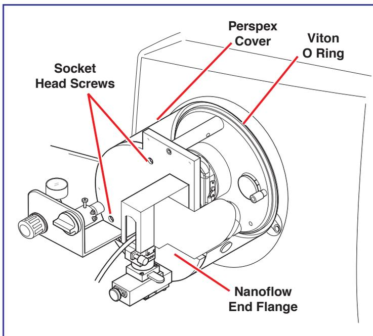
Insert the flexible light guide into the grommet at the base of the perspex cover.
