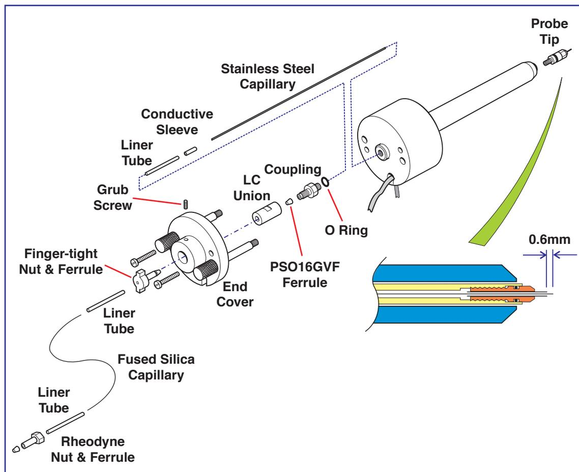
If the stainless steel sample capillary cannot be cleared, or if it is contaminated or damaged, replace it as follows:
