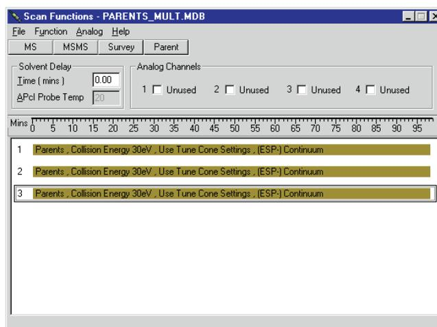
Before the experiment can be performed a file containing the required product ion, for which the precursors are sought (e.g.  $\text{PO}_3^-$ ,  $m/z$ 78.9) must be created.
