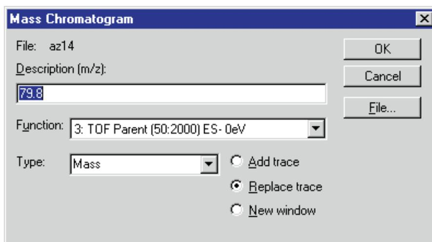
From this window display all the functions using add mode. Then using the **Mass Chromatogram** facility under **Display** in the chromatogram top banner replace each trace with the mass(es) used in the experiment.
