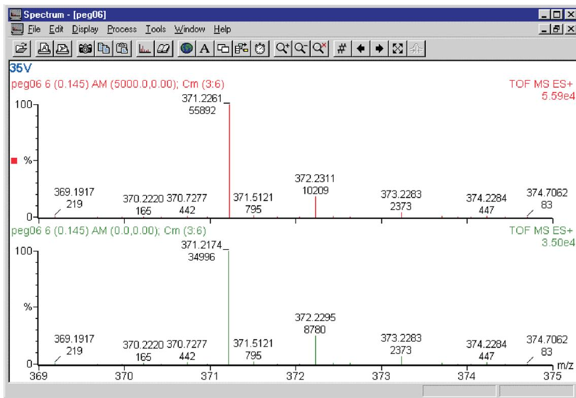
The model successfully corrects for deviations of up to about 15 mDa at mass 500, at which point the limits of the model are reached, with no correction applied at higher ion current.
