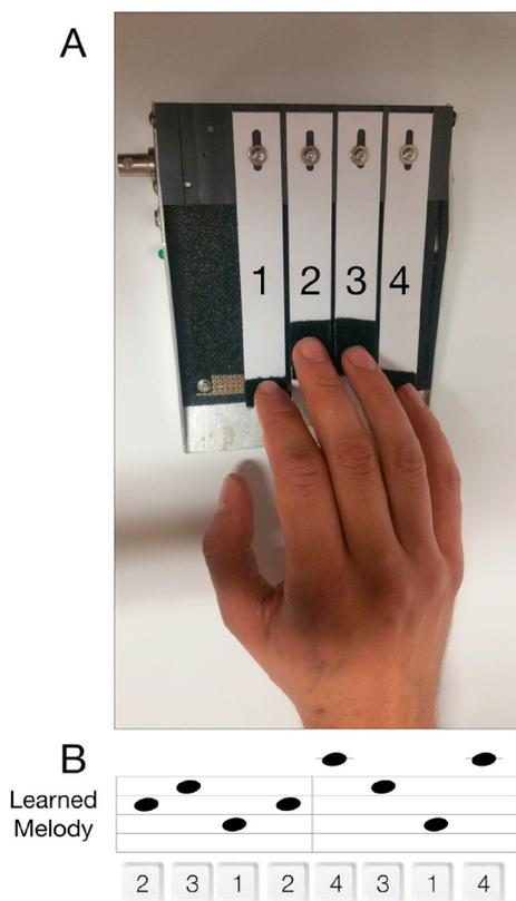
**Fig. 3.** Panel A illustrates the keyboard interface used for the experiment. Flexible plastic bars with velcro touches are depressed to actuate switches which output TTL pulses from a parallel port connected to the Beaglebone Black micro computer which recorded the key-presses. The numbers 1–4 are for illustration only to show the relationship between the keys and the sequence to be played. Panel B shows the Learned melody and the order of keys to be played on the device.
