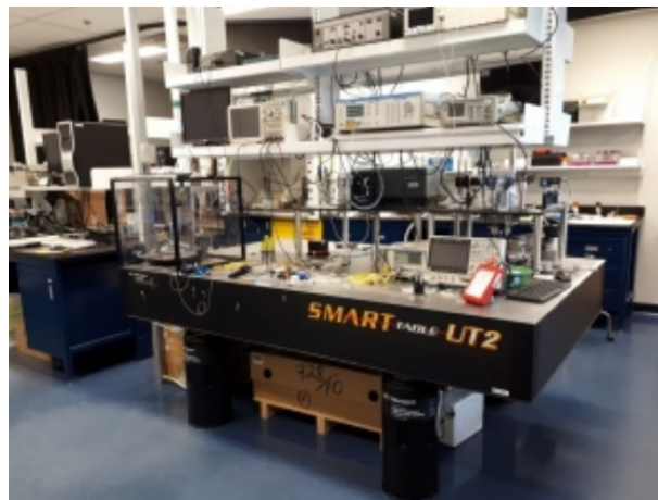
Optical Bench with vibration damping
