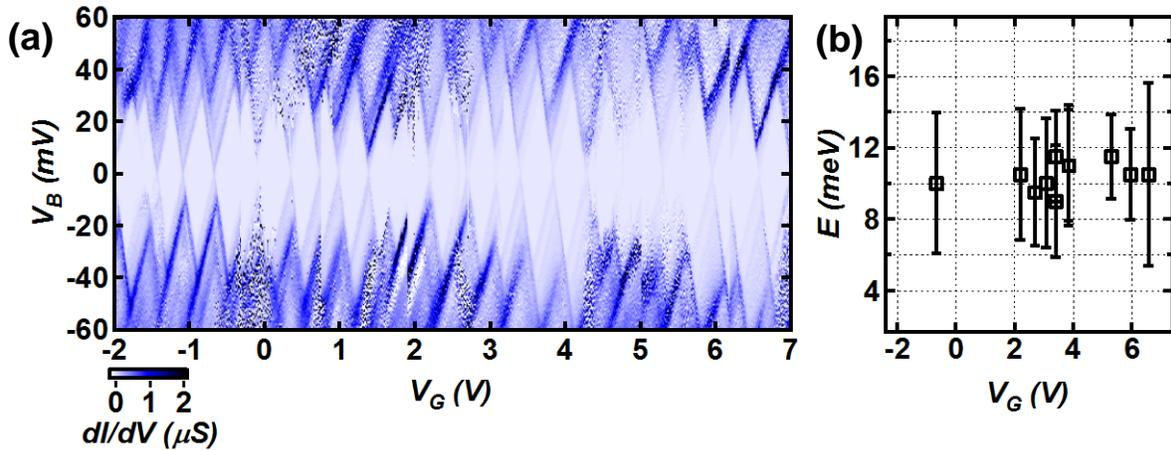
**Figure S4:** Additional data for Device B. (a) 2D  $dI/dV$ - $V_B$ - $V_G$  data (b) The vibron energies measured in (a) show no clear change as a function of the tension applied by the suspended breakjunction as  $V_G$  increases, as expected for stretching modes.
