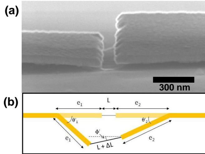
**Figure S5:** Static (built-in) strain for Device C. (a) Tilted-view SEM image of Device C taken at an angle of  $60^\circ$ . (b) Parameters used in Eq. 12 to calculate the built-in strain.
