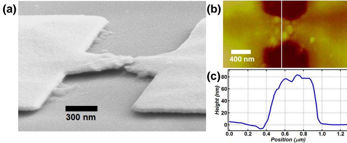
**Figure S3:** (a) Tilted SEM image of Device A taken at an angle of  $70^\circ$ . (b) 2D AFM scan of Device A. The full color scale is 200 nm, and the white line shows the position of the 1D height scan in (c). The AFM scans show a suspended height of  $35 \pm 5$  nm for the bridge, after subtracting the thickness of the gold film (40 nm).
