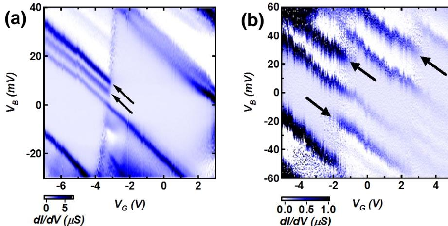
**Figure S1:**  $dI/dV$ - $V_B$ - $V_G$  data for (a) ultra-short Device D and (b) ultra-short Device E, showing the presence of stretching mode vibrons (arrows), but no bending mode resonance.
