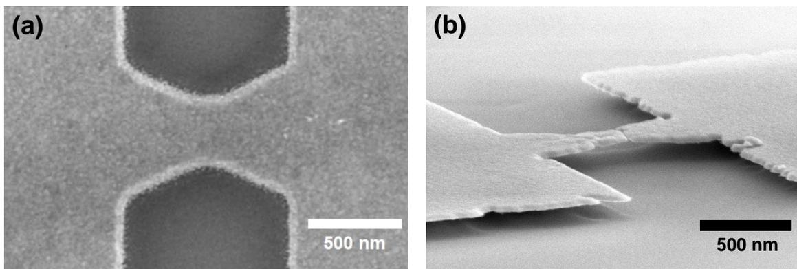
**Figure S2:** (a) SEM image of Device A before electromigration showing a constriction width of  $\approx 350$  nm. (b) Tilted SEM image of Device E showing the suspended breakjunction after electromigration.
