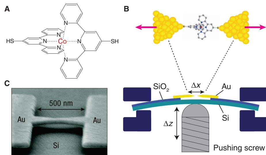
**Fig. 1.** Single-molecule electrical devices based on a transition-metal complex. (A) Chemical structure of  $\text{Co}(\text{tpy-SH})_2$ , where tpy-SH is 4'-mercapto-2,2':6',2''-terpyridine. (B) Schematic of the mechanically controllable break junction. (C) Scanning electron micrograph of a suspended break junction before molecule deposition.
