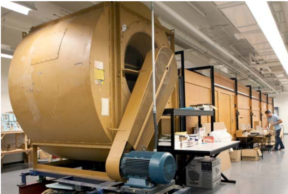
Above: The boundary layer wind tunnel (BLWT) from the back end.
