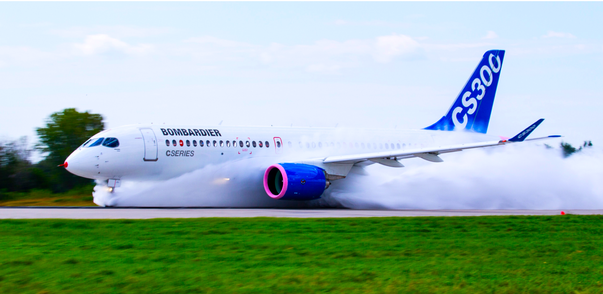
C Series Water Ingestion Test Image courtesy of Bombardier Inc.
