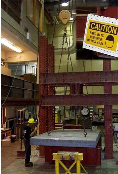
Figure 3. Technician wearing a hard hat and safety shoes during crane operations in the Structures Laboratory.
