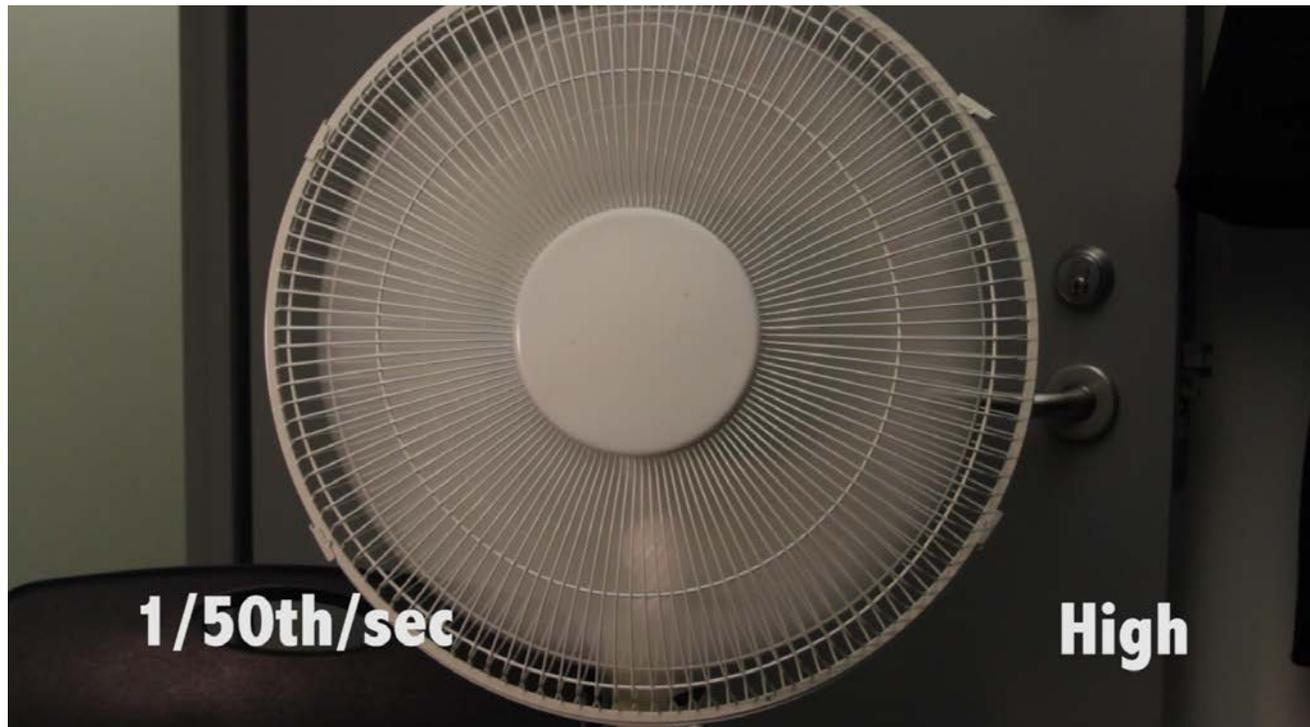
The fan is on high speed. The camera shutter speed is very high for 1080 24p video. The fan blades appear distorted. Normally all three are the same shape and size.
