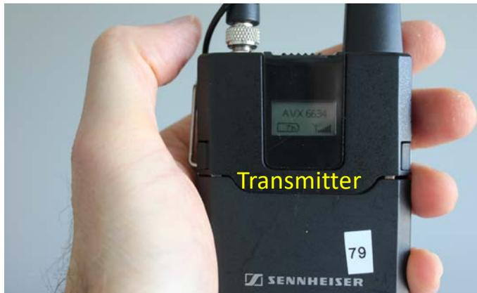
The Sennheiser AVX wireless clip-on microphone must be plugged into a transmitter.
