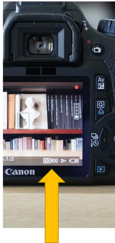
To adjust ISO, hold down the ISO button and turn the dial on top of the camera.
