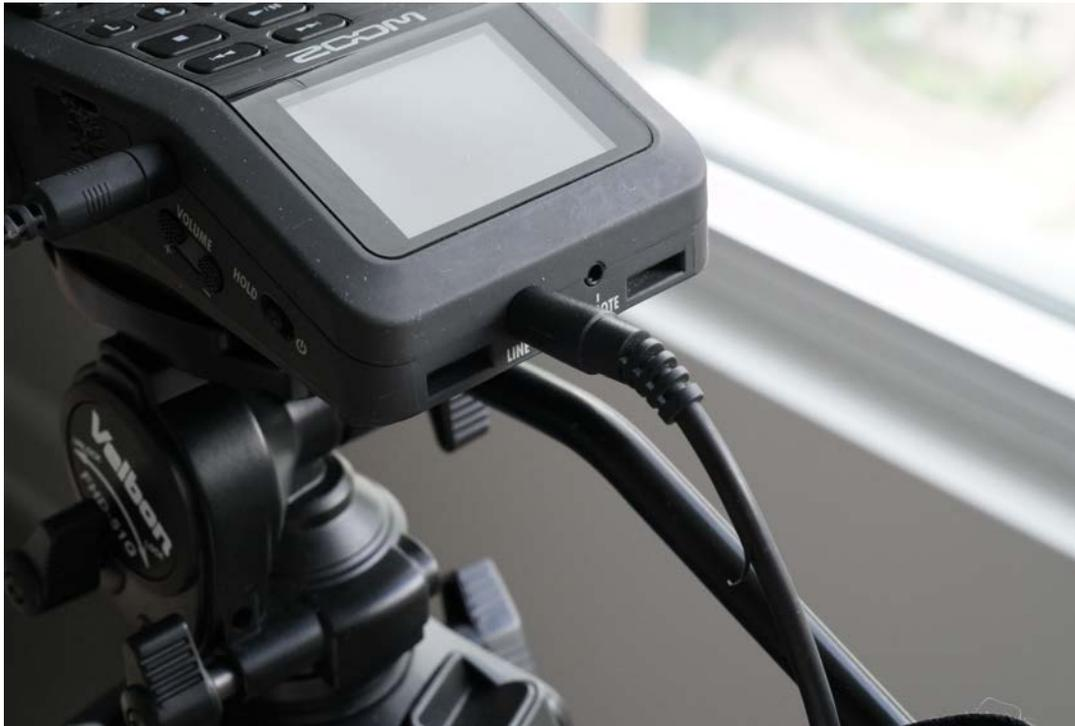
The Zoom recorder has an analog line output to send the audio signal to another device while it is simultaneously recording audio to the SD card.
