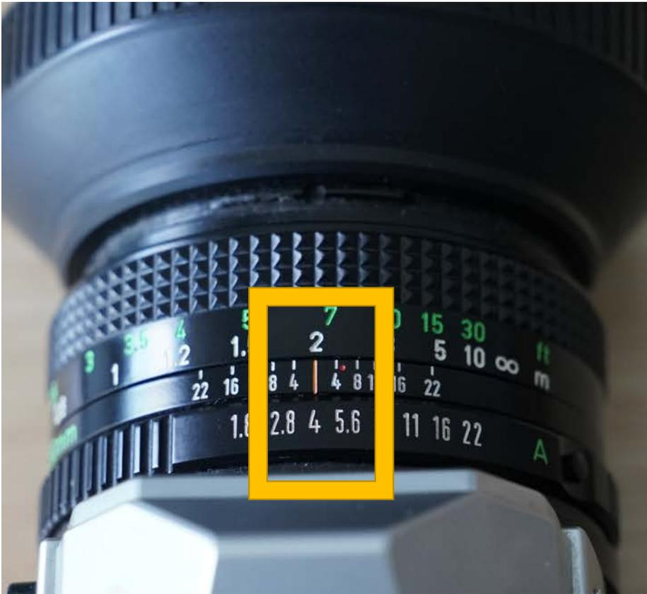
Fixed focal length lenses used to have depth of field markings on them for each aperture. Here is a lens on an older Canon film camera.
