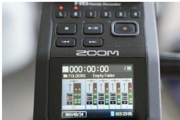
Enable the L and R buttons on the recorder. Press the R button while still pressing the L button. On the screen, the XY channel will turn red, indicating that it is ready to record. Now you can monitor your signal to see if it is loud enough.
