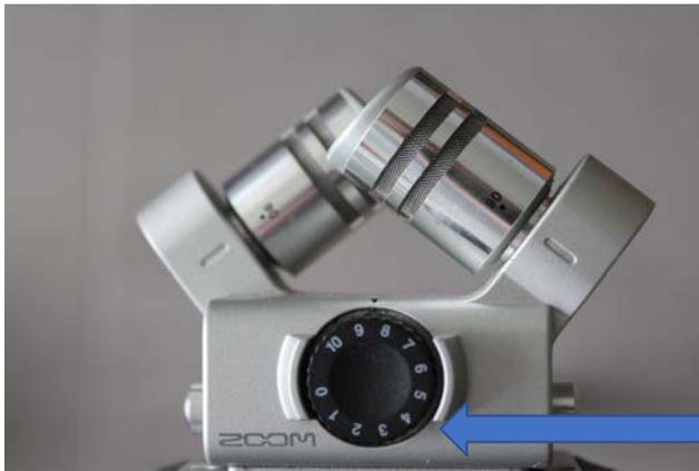
The built-in microphone is on top of the recorder. It records in stereo with two directional microphones in a XY pattern. You can adjust the width of the stereo recording from 90 to 120 degrees.
