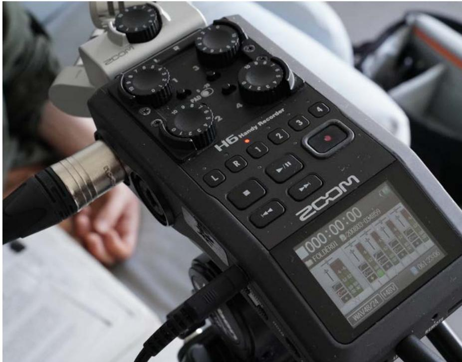
All the following microphones will plug into one of the four XLR inputs on the Zoom.
