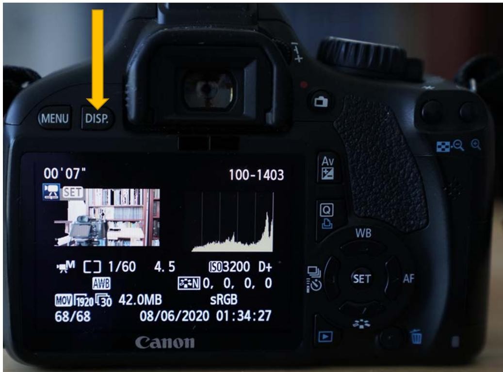
Press the display button to see an alternate display.
