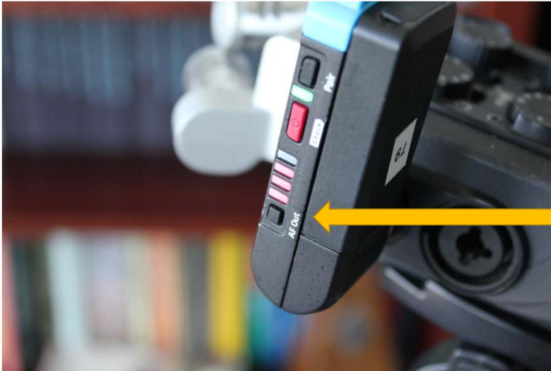
A meter on the side of the receiver shows the output volume level of the signal to the recorder.
