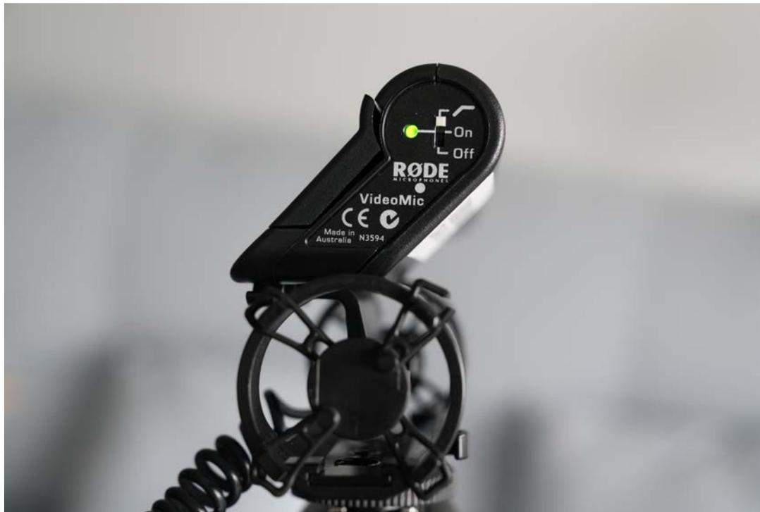
Because there are no audio meters on the LCD screen of the camera, and no indication that you are recording audio, it is very easy to plug in the microphone and to not turn it on.
