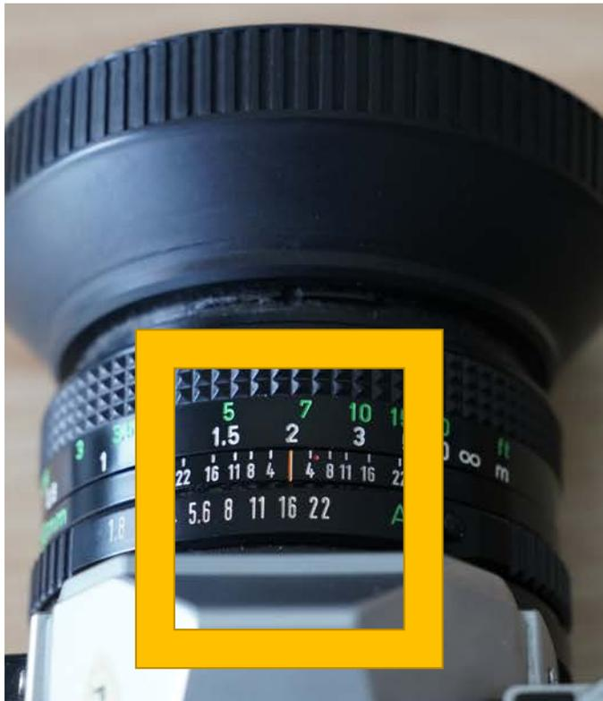
Here the markings are indicating that at f 16 the depth of field will be between 1.4 m and 3.2 m (approximately) or between 4.6 ft and 11 ft.
