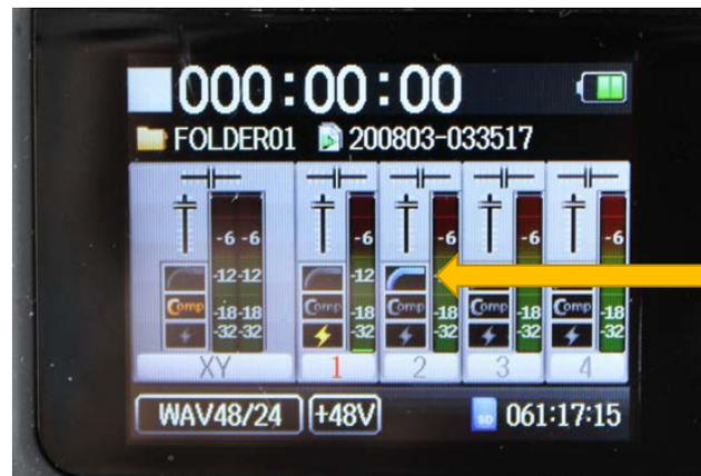
The microphone is plugged into input 2. The lo cut filter is indicated by a blue line.
