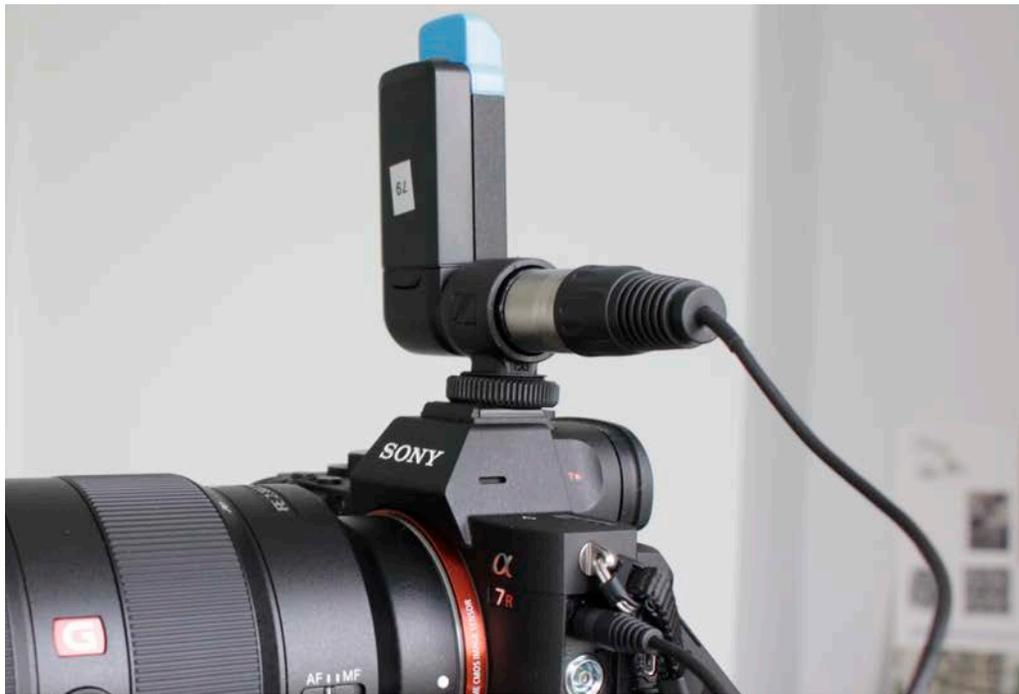
The XVX kit comes with a XLR to 1/8" adapter to plug the receiver straight into the input of a camera.
