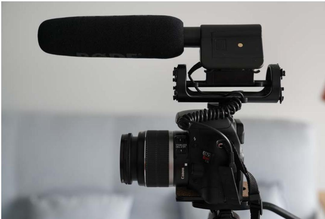
The Rode microphone is small mono directional microphone that can be mounted directly on the camera.
