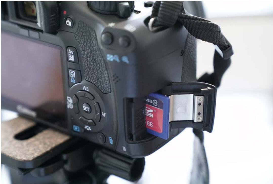
This model comes with a Class 10 8 GB SD card. This will record 22 minutes of HD video. Video can be recorded with a Class 6 SD card or higher.
