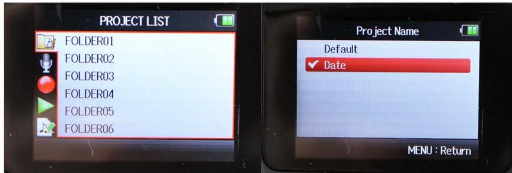
There are ten folders on the SD card. Make sure you know into which folder you are recording! Each audio file will have its own folder within that folder! The file name of the audio will indicate the channel. "LR" means the built-in microphone.
