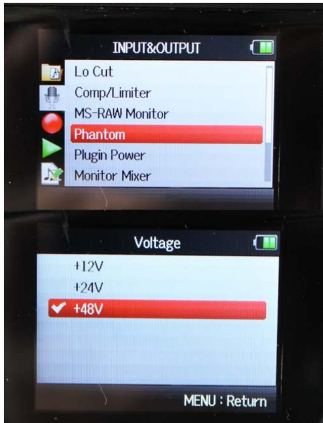
All audio devices that accept an input will have a “+48 V” button. This can be turned on to deliver “phantom power” to a condenser microphone. It should never be turned on when a dynamic microphone, like the SM58, is plugged into the channel.
