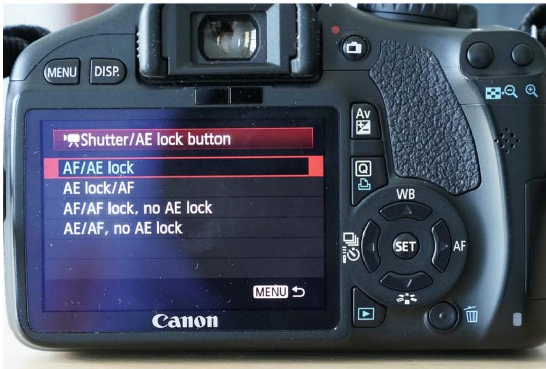
Set Shutter/AE lock Menu setting to the AF/AE lock position.
