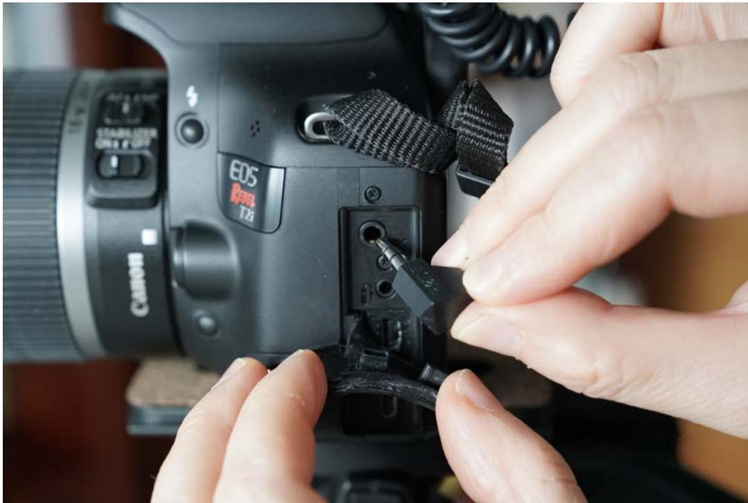
The microphone input is on the side of the camera.
