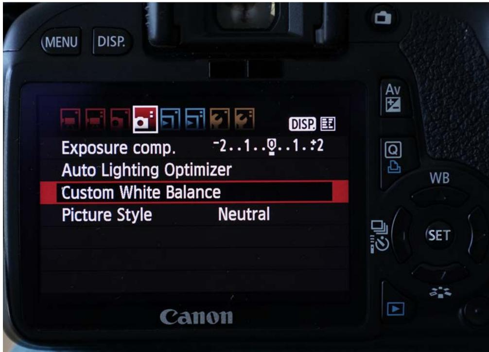
You may run into difficulties in a “mixed” lighting scenario, for example where there is a mixture of daylight and fluorescent or tungsten light. If none of the presets work, then perform a manual “custom” white balance.
