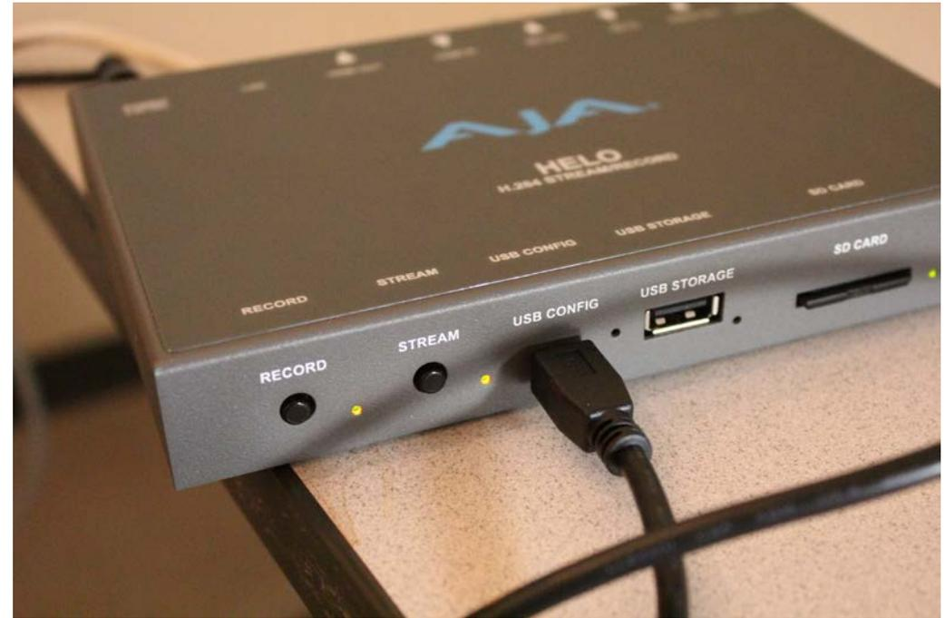
The Helo streams over Ethernet not over wireless. In general, wireless connections are not stable for streaming. Connect the Helo to an Ethernet Port, then connect it to a computer using the mini USB to USB cable provided. All of the CDA laptops have the software for the Helo installed or download it from the AJA Helo support page.
