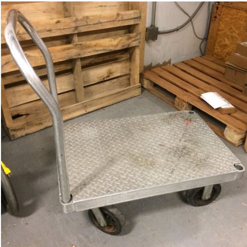
Figure 1: Example of a cart not intended for cylinder transport - Does not provide sufficient support for a cylinder - No means of securing the cylinder to the cart
