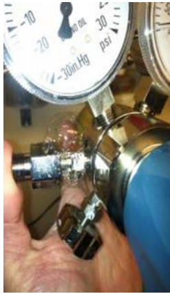
Figure 12.5.1: Leak test on gas cylinder valves. (ref: pubs.usgs.gov)
