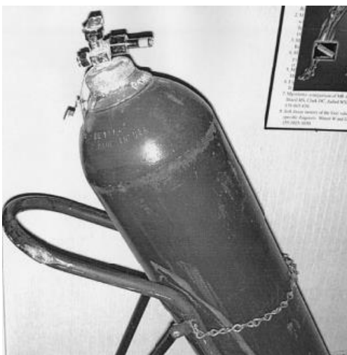
Figure 15.1.1.1: Damages from impact between an oxygen cylinder and MRI instrument. (ref: Colletti, P. M., J Magnetic Resonance Imaging , 2004, 19, pp. 141-143)
