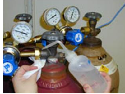
Figure 12.5.1: Leak test on gas cylinder valves. (ref: pubs.usgs.gov)
