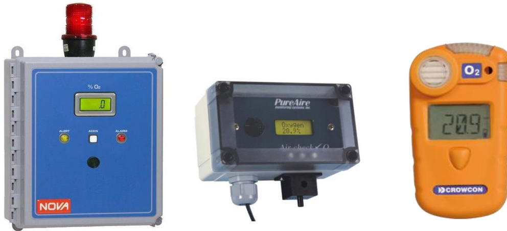
Figure 5.5.1: Fixed or portable oxygen monitoring alarm devices. (ref: www.directindustry.com ; www.pureairemonitoring.com ; www.pce-instruments.com )
