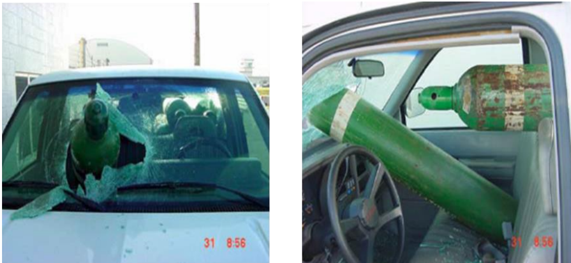
Figure 13.3.2.2: Improper transport of compressed gas cylinders. (ref: Messer France S.A.S., Transport de gaz dans des véhicules non ADR)
