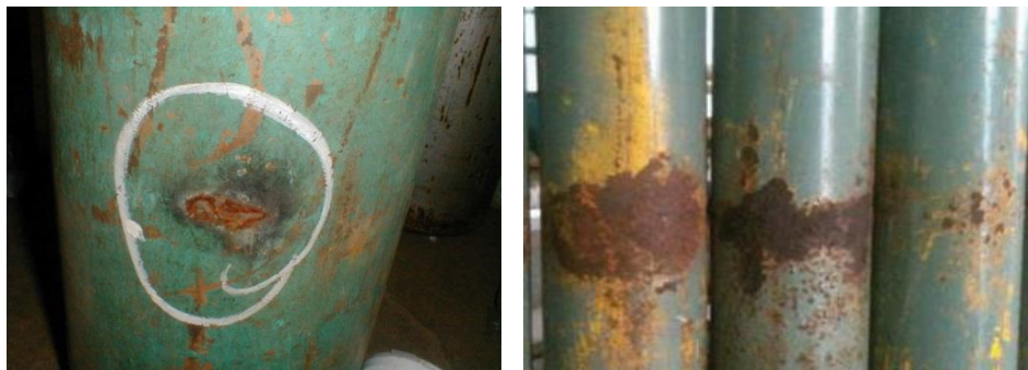
Figure 5.7.1: Cylinders showing arc and corrosion damage (ref: www.engineeredinspection.com ; www.nautinst.org )
