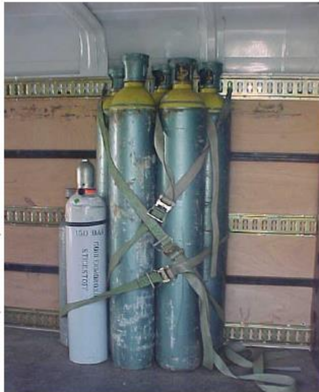
Figure 13.4.2.1: Proper cylinder load inside closed vehicle. (ref: Messer France S.A.S., Transport de gaz dans des véhicules non ADR)
