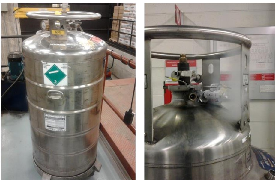
Figure 6.9.1: Liquid cylinder (Dewar) with pressure-control relief valve exhausting excess gas (ref: Concordia University)
