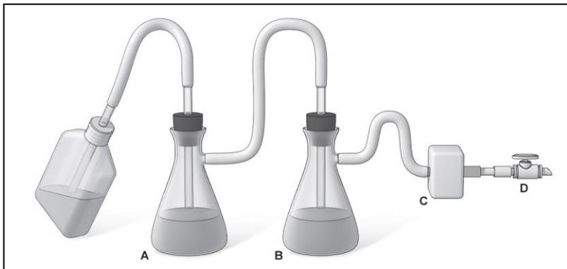
**Figure 1:** Flask (A) collects the contaminated fluids into a suitable decontamination solution; flask (B) also contains a suitable decontaminant and serves as a fluid overflow collection vessel. An in-line HEPA or 0.2 µm filter (C) protects the vacuum system (D) from aerosolized microorganisms or toxins.
