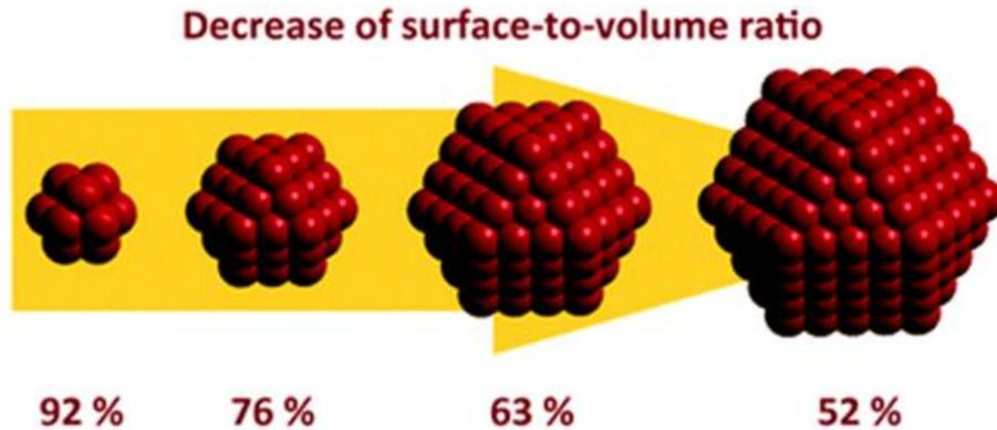
**Figure 8: Surface-to-volume ratio of nanoparticles**
