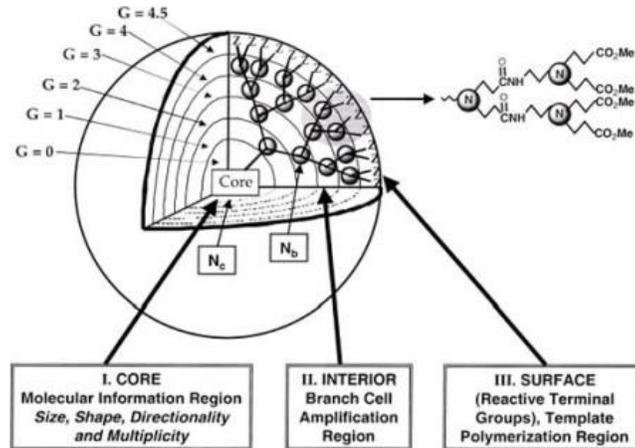
**Figure 6: Dendrimer engineered nanoparticles**
