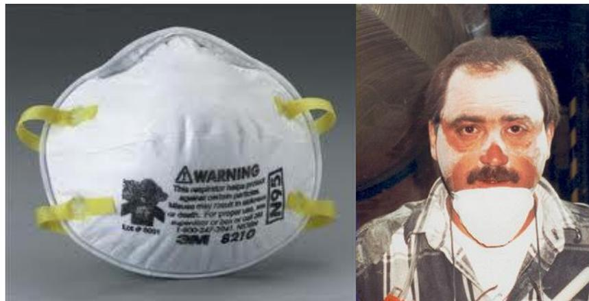
**Figure 23: N95 FFR with an improper use of mask: the white powder around the nostrils shows that this mask did not have a tight fit.**
