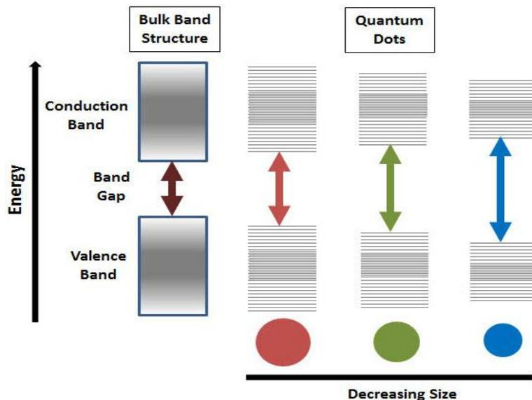
**Figure 9: Quantum effects of size reduction of nanoparticles**
