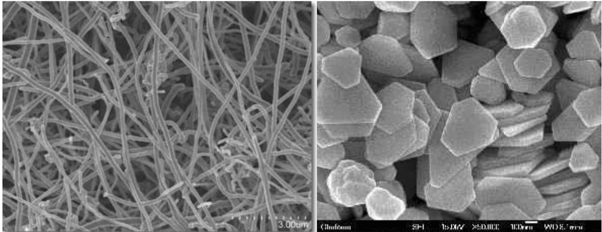
**Figure 2: Carbon nanofibers (left) and silver nanoplatelets (right)**
