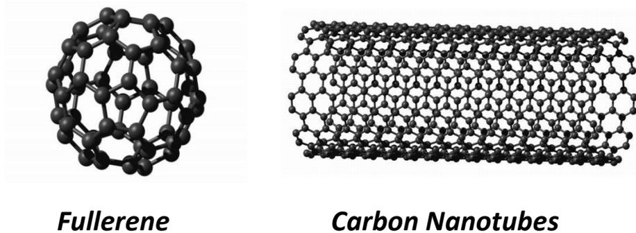
**Figure 4: Carbon-based engineered nanoparticles**
