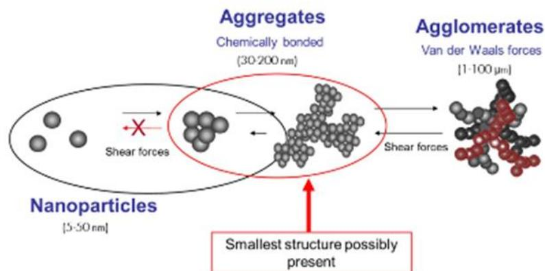
**Figure 3: Nanoparticle aggregates and agglomerates**
