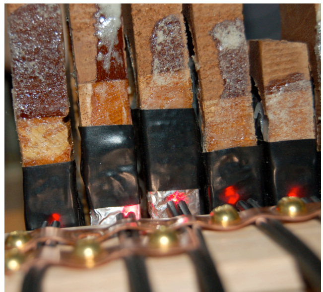
Figure 1. Optical sensing of piano key movement.
