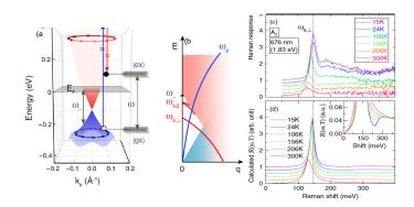
Demonstration of application of our theory for collective mdoes applied to topological insulator Bi<sub>2</sub>Se<sub>3</sub>. (a) Electronic states on the surface of the material. (b) The dispersion of the exotic chiral-spin modes. (c) Experimental data for the intensity of the Raman signal. (d) Theoretical calculation of the Raman intensity. Figures from PRL 119,136802 (2017).
