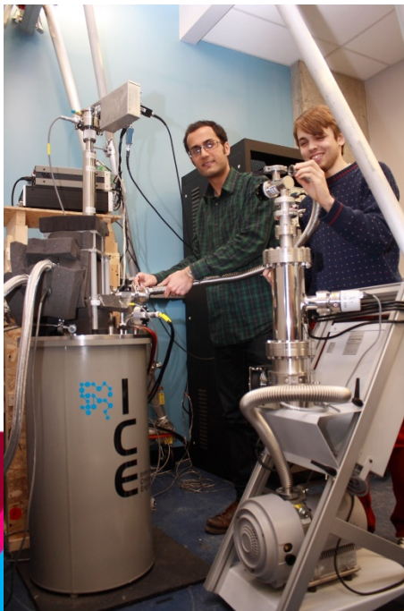
Cryostat for transport measurements
