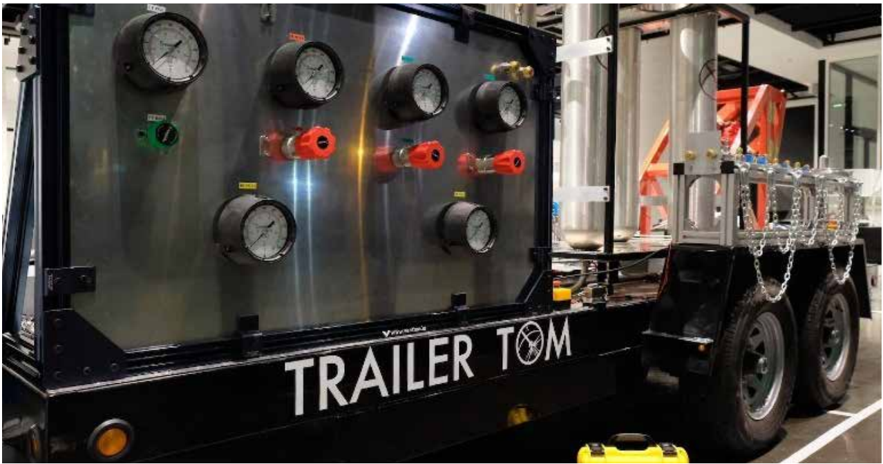
Inspired by a David Bowie song, Trailer Tom is the mobile rocket-engine test stand built by Space Concordia using materials and equipment from Swagelok Québec's $37,000 gift-in-kind
